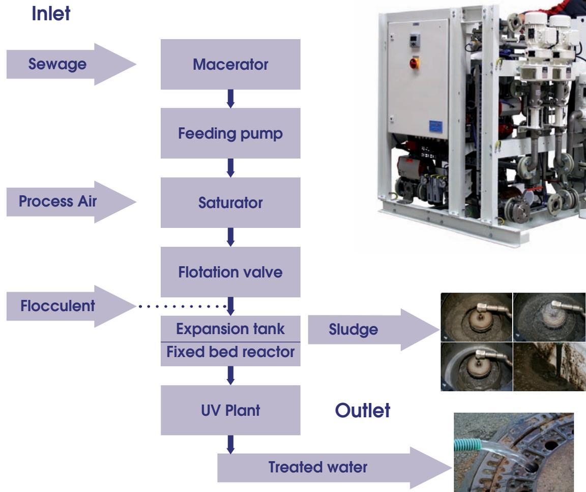
All sewage needs to be collected in one ship's holding tank. Depending on the calculated load and number of persons the tank must have a sufficient size as the working volume between high level and stop plant is one important issue for the HL Cont PLUS.
